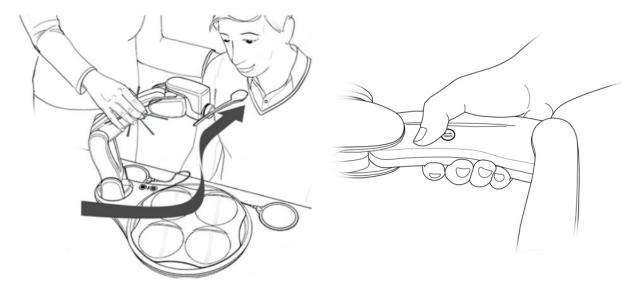
When the Teach Icon is covered, the Arm will be free for the caregiver to move. The last two sections of the Arm will remain engaged and will keep the Spoon level when moving within the teach space. If resistance to movement is present, the thumb is probably not completely covering the Teach Icon.
